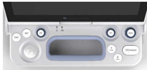
Fig. 3 The SONIMAGE HS1 control panel. All major functions are controlled with only 8 buttons and a trackball.
